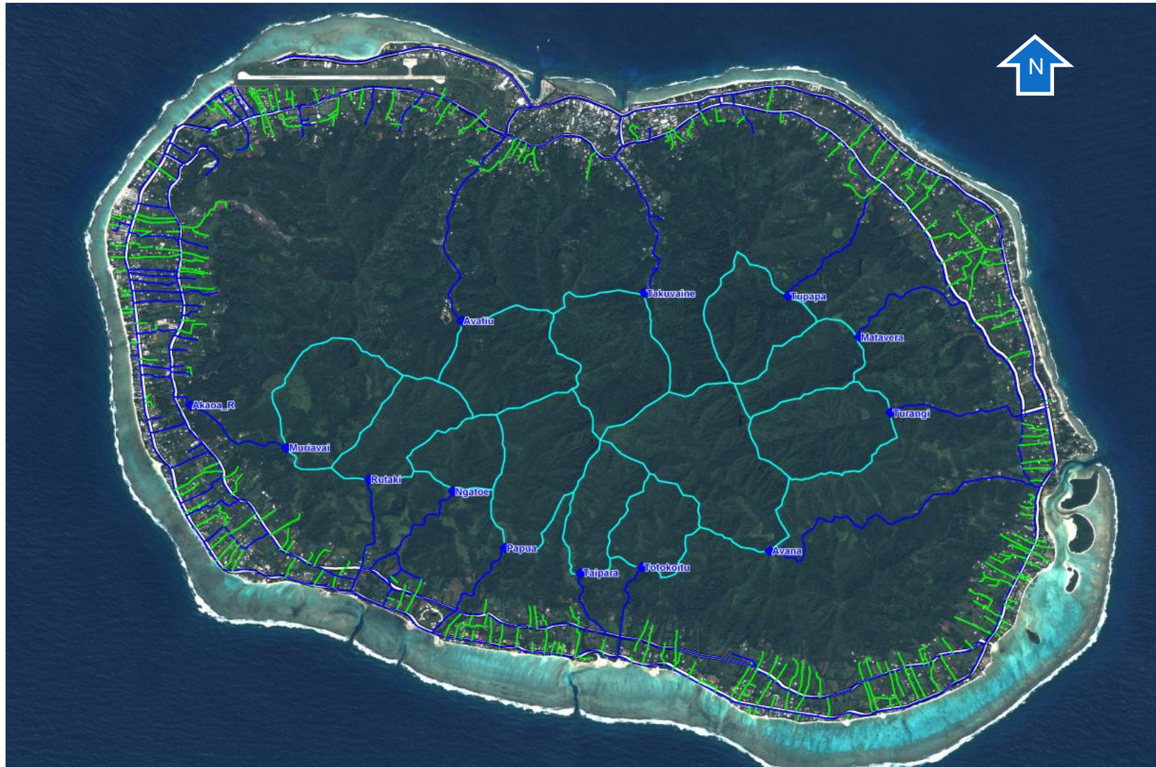
Figure 13 - Rarotonga Water Supply Network showing the 12 water intakes (and water catchments) and the Reservoir (Source: Infrastructure Cook Islands, 21/01/14)
